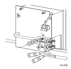
4. Attach the grounding cable to the ground lug on the power supply.
